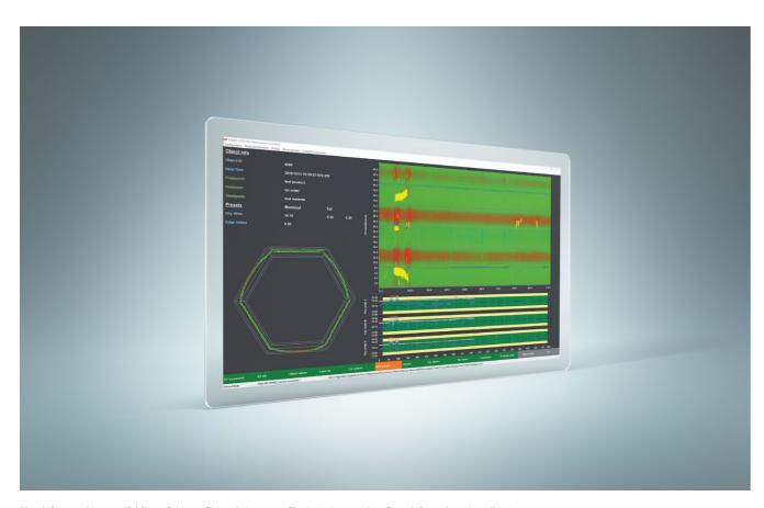
The defect card is an unfolding of the profile and shows profile deviations and surface defects (here in yellow).
