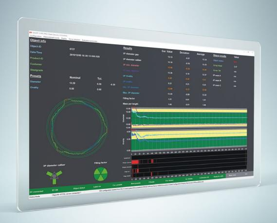
A typical screen for users: the green of the icons to the lower left shows that all measured values used to identify rolling faults are within tolerances.
