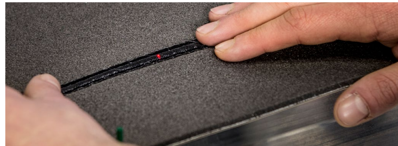
The spot lasers mark the course of the decorative seam at multiple points on the back of the decor. This enables fast, precise positioning.
